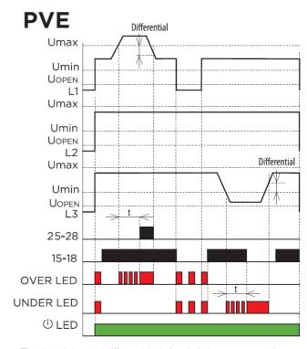
The time delay and differential trip levels help to prevent relay chatter as the monitored voltage level varies.
