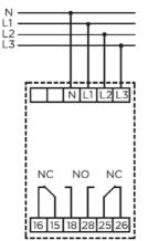
NC = Normally closed. Contact closed when relay de-energised.
